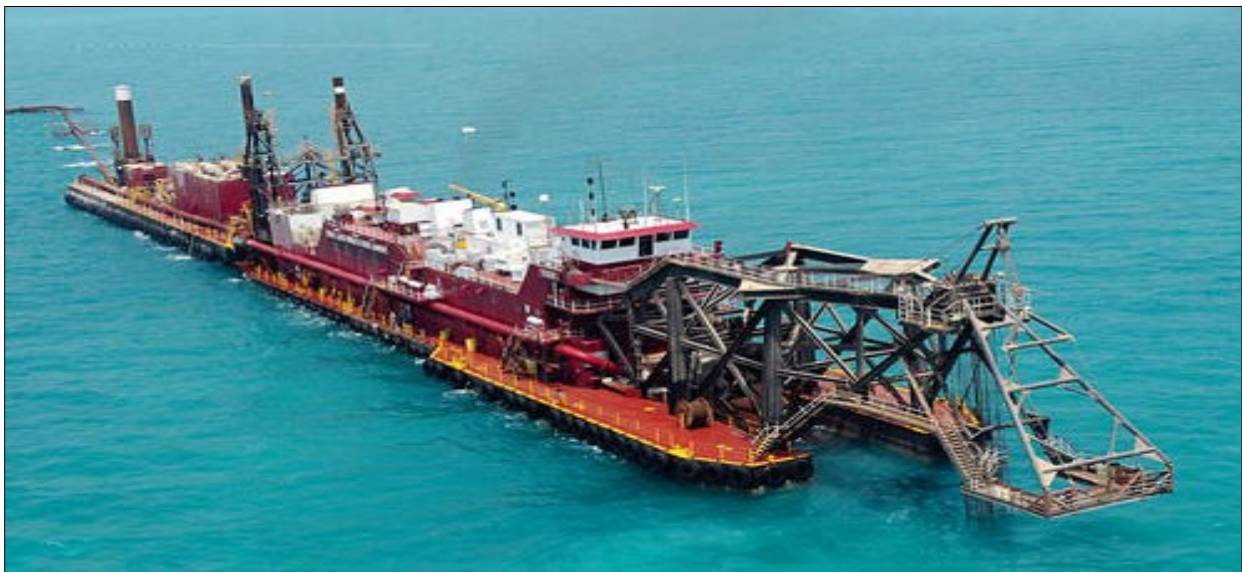
Figure 6-2. Typical Hydraulic Cutterhead Dredge Plant.
